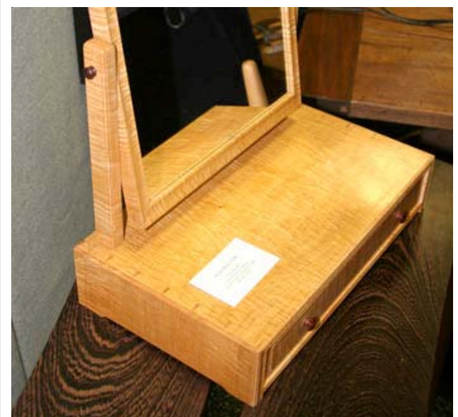
Delicate details. The judges admired the tiny dovetails, refined pulls, and surface treatment of this bureau mirror by Josh Metcalf.
